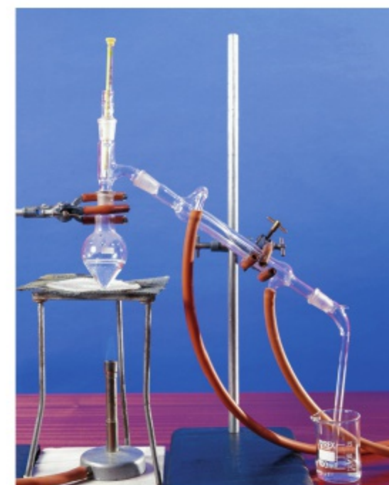
▲ fig B This is just one of the many apparatus set-ups using ground-glass joints.
